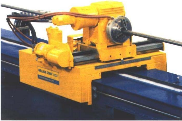
Fig. 2 The carriage on a Jesse Engineering 1000-PC series bender incorporates powered centerline radius adjustment, for ease of set up, and offers two chuck or collet options - to best meet your bending needs.
