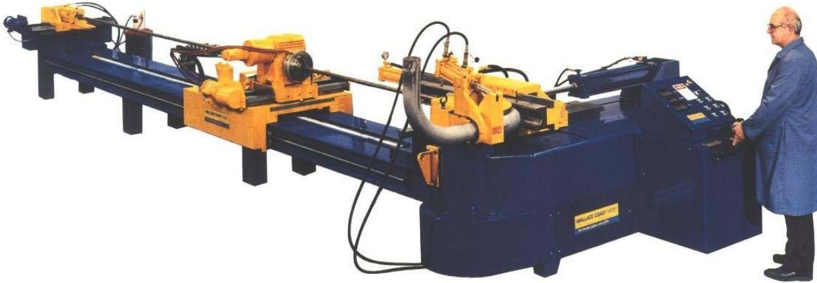
Fig. 1 A Jesse Engineering 1004-PC powered carriage bender - 4" Sch. 80 IPS capacity (114 x 8.5 mm). 20'-0" load length is standard on all Jesse Engineering 1000-PC series benders.
