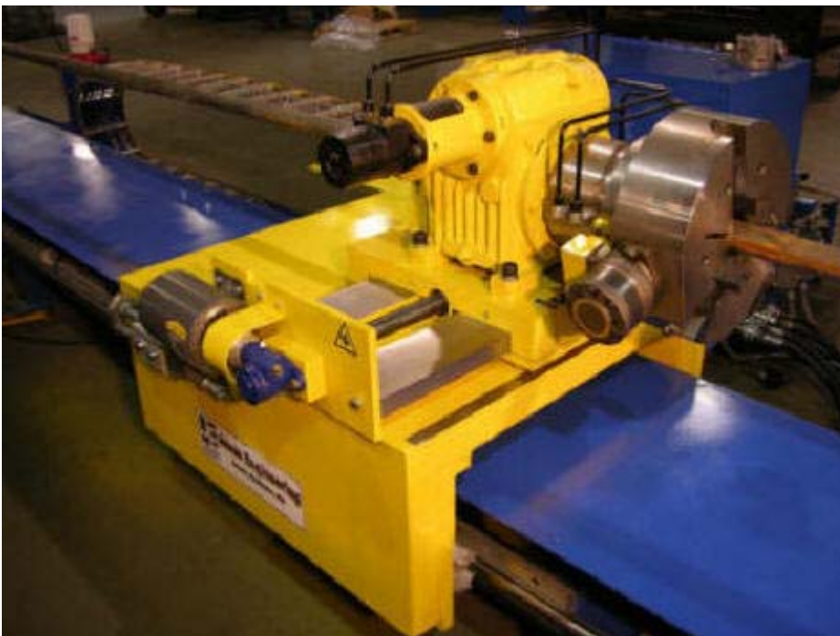
Fig. 3 Power centerline radius adjustment of the carriage and the mandrel unit during set-up is standard on 1000 CNC series benders.
