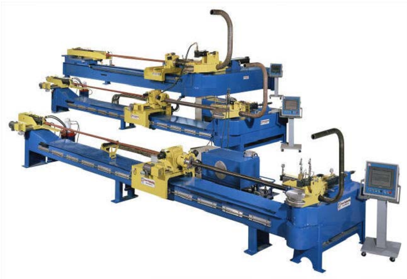
Fig. 1 Jesse Engineering CNC Pipe Benders. 20' load length is standard.
