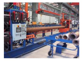
The FW360MTAW is a complete semiautomatic pipe flange welding system. Pipes of varied length from 1-1/4" to 14" nominal diameter roll into the machine. Pre-loaded slipon flanges are then manually tack welded onto the pipes. Four automated weld heads are lowered down onto the tack welded pipe spools. Four fillet welds are applied simultaneously. Automated loading tables and unloading carts are normally available as options.
