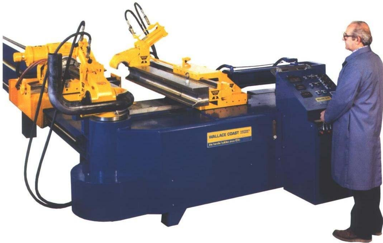
Fig. 4 The "overhead clamp" on top of the radius die opens out of the path of the advancing workpiece. This machine is a booster bender with a second clamp - the booster clamp - on the rear of the pressure die. Booster bending permits right radius bends with a minimum of wall thinning.
